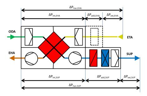
The **specific fan power**, *SFP*<sub>int</sub> is the electric power supplied to a fan and related to the internal pressure of all ventilation components (Filters, heat recovery and related casing including flow entrance and exit) divided by the air flow expressed in m<sup>3</sup>/s under design load conditions.
