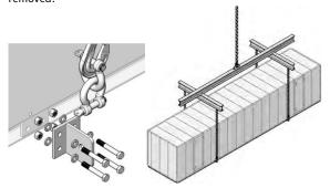
Maximum permissible weight load per module 5000 kg (light version) or 8000 kg (heavy version)
