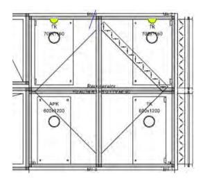
Here, too, the joints between the plate heat exchanger and the housing must be sealed with sealant after assembly.
