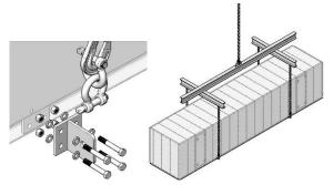
Maximum permissible weight load per module 5000 kg (light version) or 8000 kg (heavy version)
