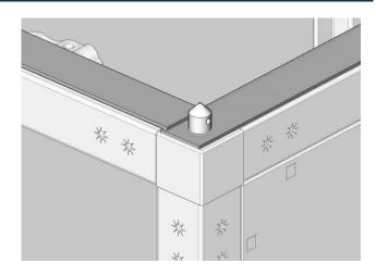
For unit widths between 2000 and 3000mm, the supplied trough connectors (see diagram) must be fitted on site.
