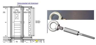
Split modules over 600kg are to be transported with the help of lifting slings.
