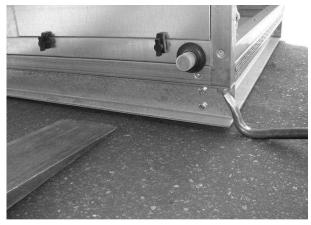
The maximum load capacity of the forklift truck must not be exceeded when transporting the modules. If the unit is equipped with a sheet metal base frame, the fork carrying width of the forklift truck must be at least 1310 mm in order to be able to use the transport openings provided.
