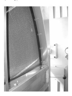
As a matter of principle, the bearing of the rotor is aligned in the factory. However, depending on the installation conditions, a realignment may be required. Please refer to the manufacturer's operating instructions.
