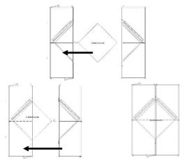
Do not use the pre-assembled unit connectors to pull the modules together! These can tear out or deform the unit if overloaded. After connecting the unit parts, check the position of the heat exchanger in the holding rails again and readjust if necessary. Once assembly is complete, grout the unit joints and corners.
