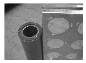
To ensure proper functioning of the filter cartridges, an odour test must be carried out after the filters. If necessary, replace the cartridges.
