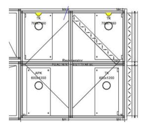
Here, too, the joints between the plate heat exchanger and the housing must be sealed with sealant after assembly.
