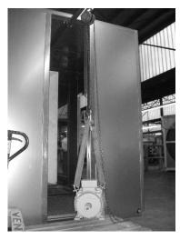
The roller and chain hoist are to be installed for maintenance purposes only and must be removed upon completion of the work. They must not remain in the unit during ventilation operation. The pull-out rail, roller and chain hoist must be inspected regularly in accordance with DGUV V54 (Winches, Hoisting and Pulling Equipment).
